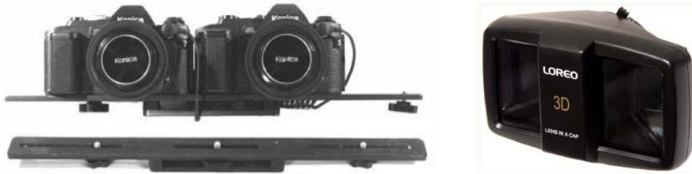
Figure 2. Two cameras mounted side by side and an example of a beam splitter.
