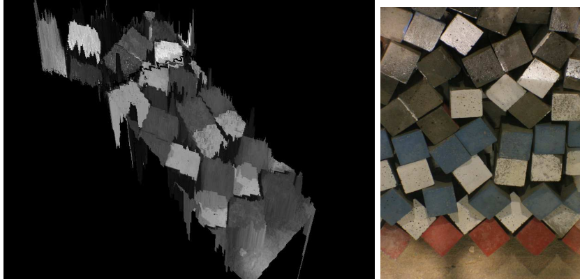
Fig. 7. 3D view and left image of another model breakwater partially submerged.
