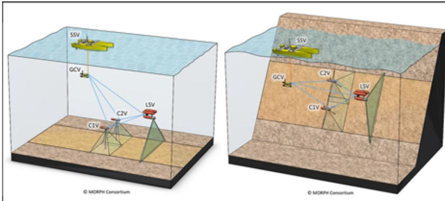
and recognizing the environmental situation and triggering the formation adaptation. This detection is done both with a forward-looking scanning profiling sonar, but also a MBES used to estimate the relative angle of the survey surface. This angle is relayed to the following camera vehicles, which they use to modify their relative position setpoint in the formation. Figure 1b shows the MORPH Supra-Vehicle adapted to a MORPH-Roll-Angle of 60° in an idealized graphic.
