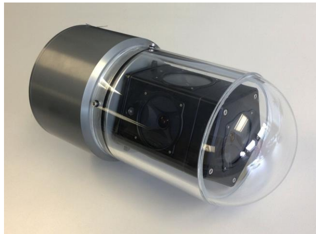
Figure 2- Omnidirectional sensor based on a 6-camera system. A custom housing was designed and built, comprising a cylindrical viewport with a hemispherical cap, and a metal container for a small form factor pc.
