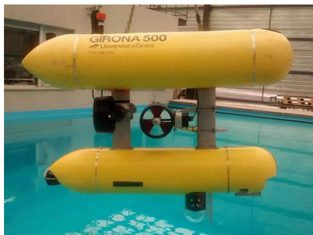
Figure 3 - Side view of the Girona 500 AUV/HROV with the omnidirectional camera installed.
