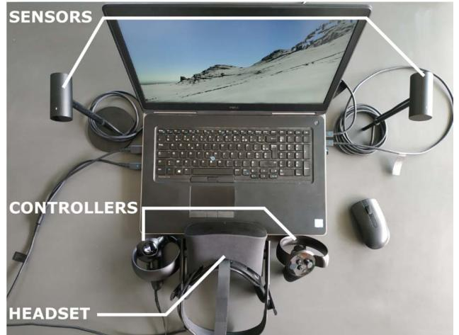
Fig. 1. Oculus Rift headset with two sensors used for localization and the two Oculos touch controllers. The Oculus Rift S is similar except that it use embed camera for headset localization instead of external sensors.
