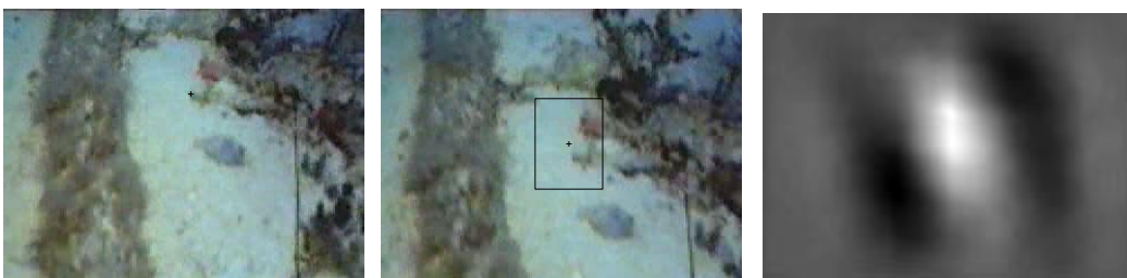
FIG. 1. Search area selection: image I_1 (left) with selected feature, search area on I_2 (center) and cross-correlation image(right)
