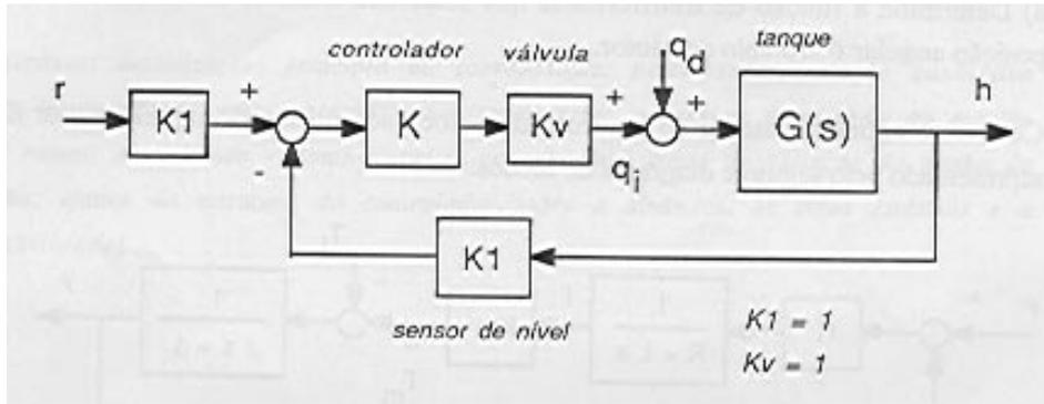
a) Determine  $G(s)$  para  $A = 4m^2$  e  $R = \left. \frac{dH}{dQ_0} \right|_P = 1m^{-2}s$ .
