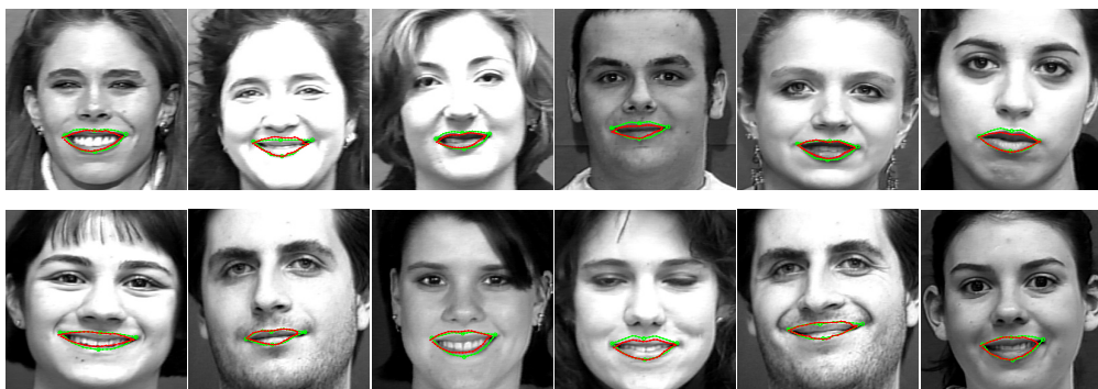
Fig. 17. Test lip sequences displaying the “happy” expression. The ground truth (in green) is superimposed with the segmentation results (in red).
