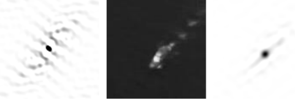
Fig. 3. From left to right, the correlation filter \alpha trained and updated throughout 226 frames, the candidate patch for detection z after 227 frames since the initialization, and the response map \bar{y} . Using the trained correlation filter it is possible to estimate the translation of the target relative to the previous position.
