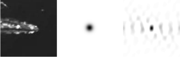
Fig. 2. From left to right, the region of interest x , the desired output as a 2D Gaussian y and the corresponding correlation filter of the first frame, assuming the use of raw image pixels as features, obtained using Eq. (16) and a Gaussian kernel.
