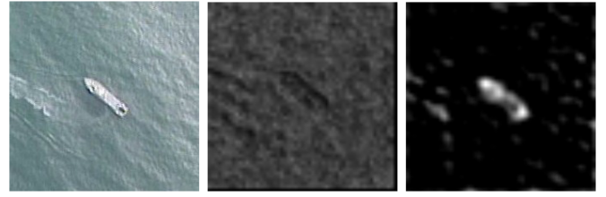
Fig. 4. From left to right, original image, one channel of the FHoG features from a total of 31 and one channel from the CNN features from a total of 256 channels.
