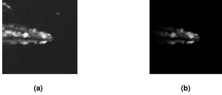
**Figure 3.3:** (a) Grayscale of the original image patch of a vessel to be tracked. (b) Image patch of the target weighted with a Hanning window, Eq. 3.75 and Fig. 3.2(b). Note that the focus of the image is on the target and the boundaries are smoothly converging to zero which attenuates the image boundary discontinuities that affect the DFT.
