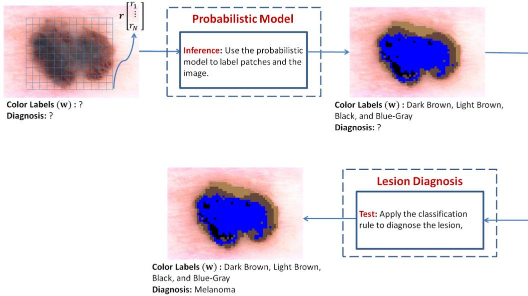
**Fig. 4.** Proposed framework: test step. Here  $\mathbf{r}$  is the collection of local features  $r_n$  and  $\mathbf{w}$  represents the corresponding global text labels.
