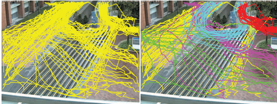
Fig. 1. (Left) Detected trajectories in UPC campus, (right) the same set of trajectories, but each trajectory has a different color label according to the trajectory-class (activity). In this scenario the following classes are considered (see right image): a_1 \rightarrow walking and stepping down the stairs, (magenta); a_2 \rightarrow walking along, (yellow); a_3 \rightarrow crossing and stepping down the stairs, (green); a_4 \rightarrow pass diagonally, (red); a_5 \rightarrow turning the campus (cyan).
