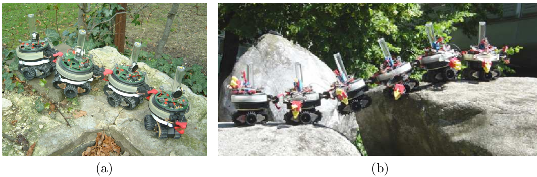
Figure 1: A group of robots physically connected to each other, that (a) moves on rough terrain; (b) passes over a gap. These pictures are demonstrative of the capabilities of the self-assembling robots we developed.
