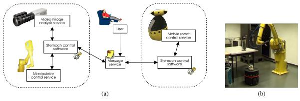
Fig. 2. Software architecture of the coffee serving system (a), and the system at work (b).
