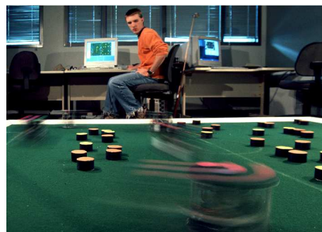
Fig. 1. The robotic system in action. Initially designed to play robot soccer [15], it can monitor and control up to 8 robots.
