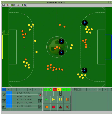
Fig. 4. The main system monitor has the ability to take control of all the robots in the system either separately or as a group. More importantly a single user has the ability to monitor the entire system from a single PC using the system monitor.
