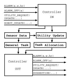
Fig. 2. Generalized Node Architecture.
