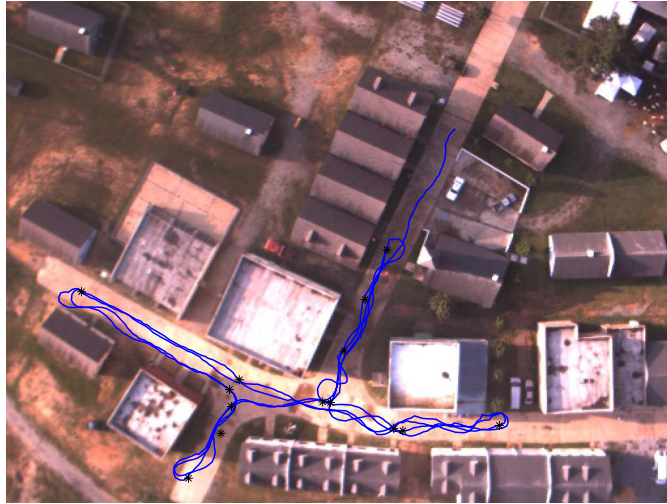
Figure 2. Trajectory of a robot navigating using a sequence of waypoints. The waypoints are depicted as ‘*’ and the robot executes the sequence twice.
