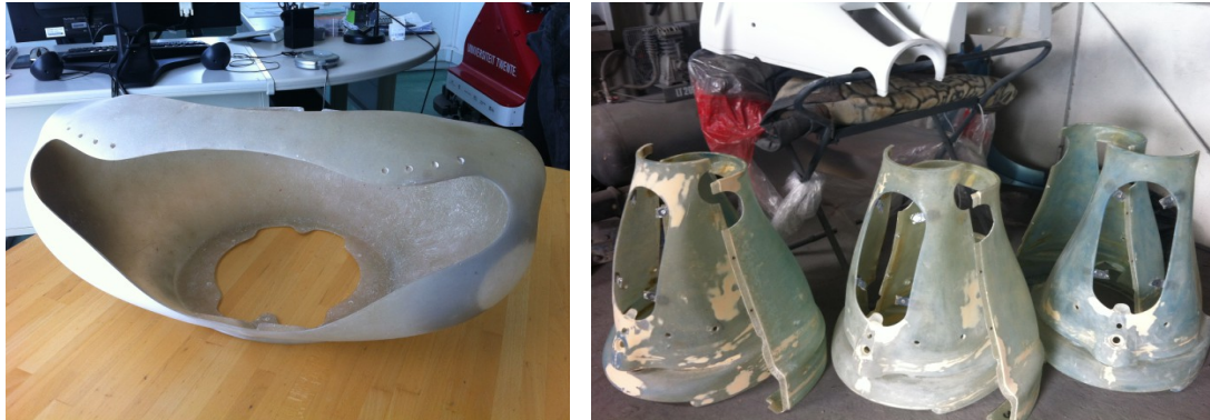
Figure 39: production of the shell
