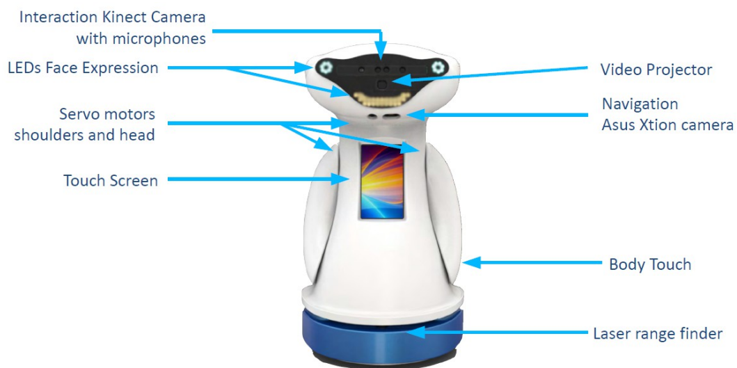
Figure 29: location of onboard devices
