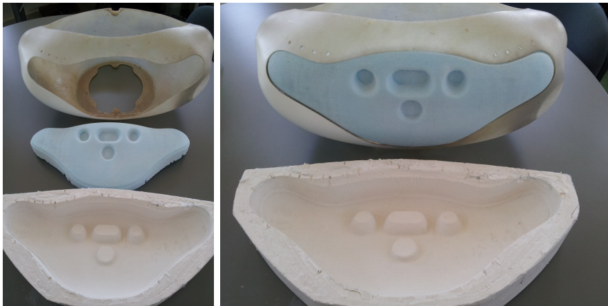
Figure 42: making the mould for the visor (i)
