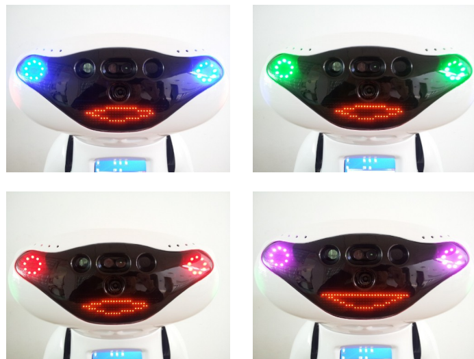
Figure 14: MOnarCH RGB LED eyes and mouth dot-matrix LEDs
