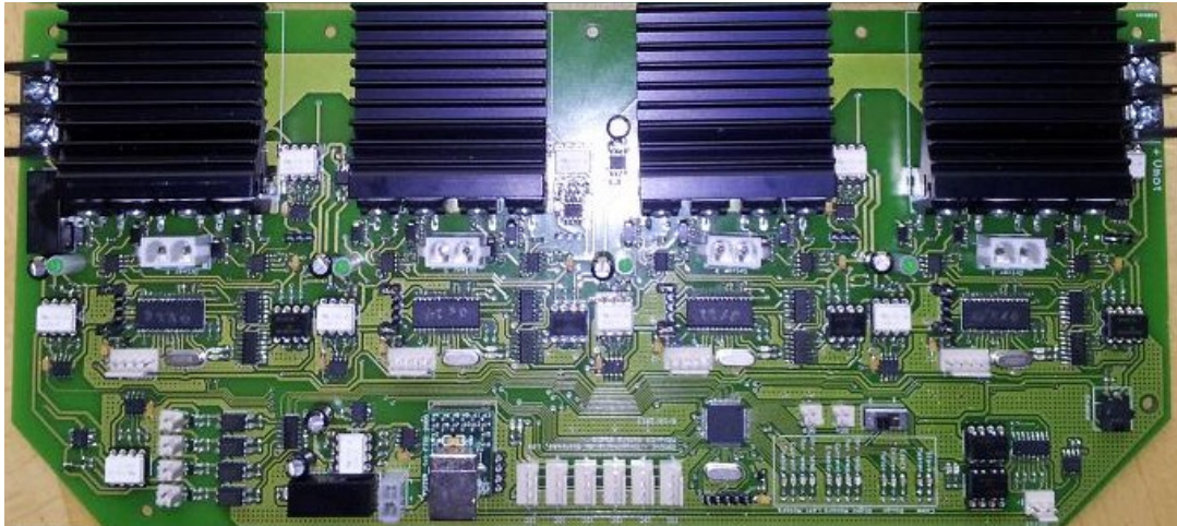
Figure 52: Motor Controller Board
