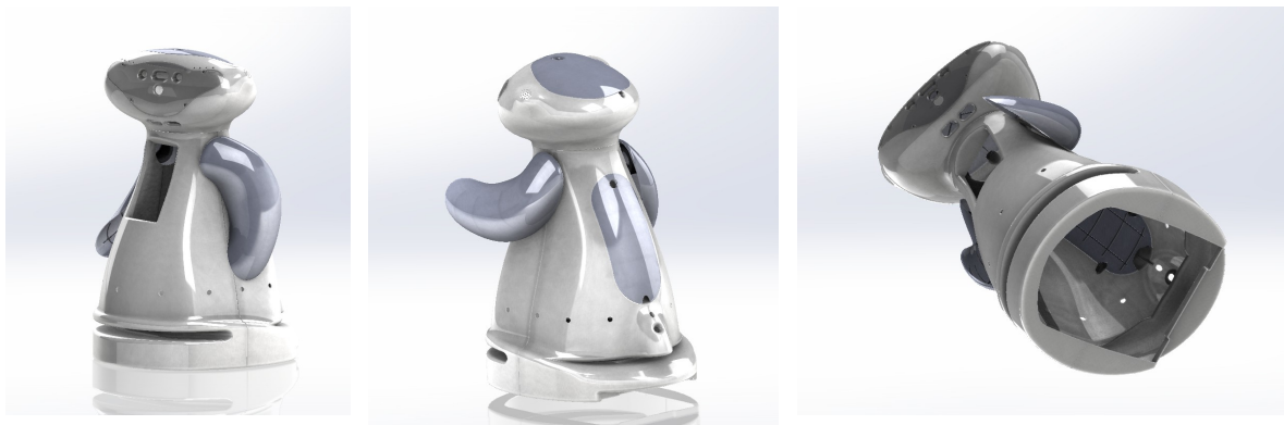
Figure 35: design of the shell for production
