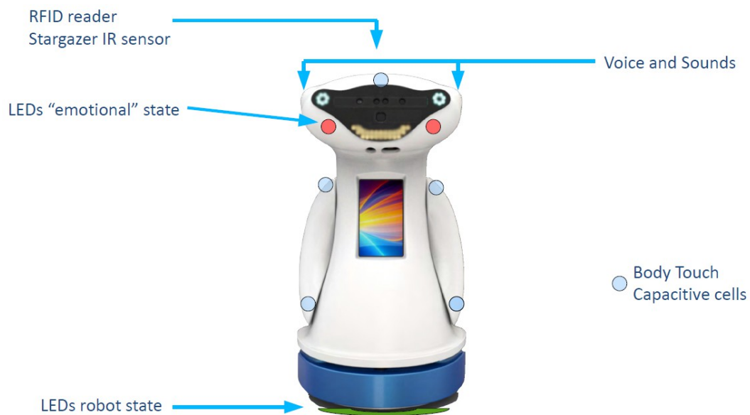
Figure 30: location of onboard devices (cont.)
