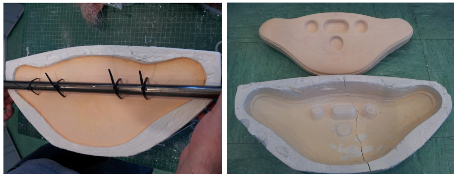
Figure 43: making the mould for the visor (ii)
