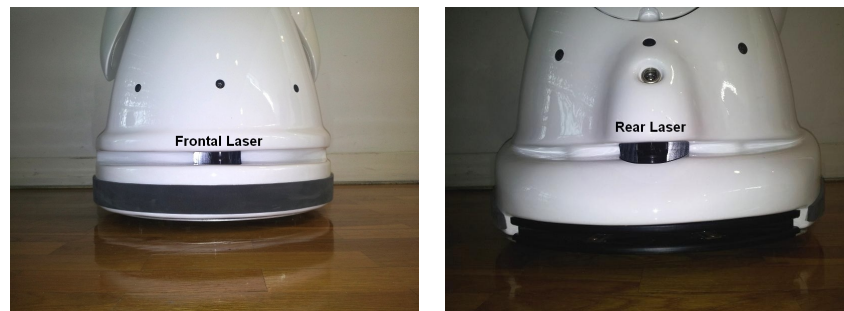
Figure 5: MOnarCH LRFs. Left picture: front LRF. Right picture: rear LRF
