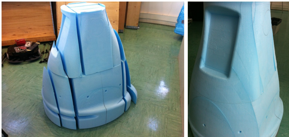
Figure 37: putting the drilled parts together for the body mould
