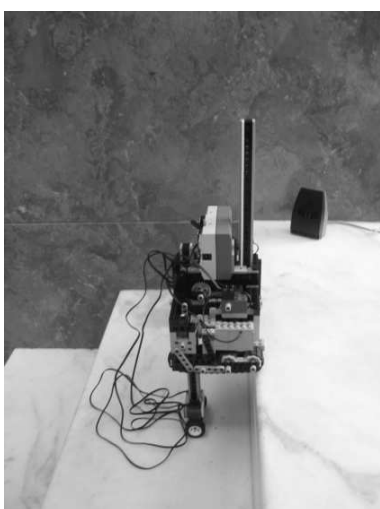
Figure 12. Retracting frontal wheeled-leg
