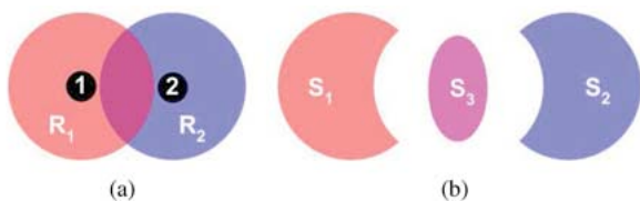
Fig. 5. (a) Sensing regions of two sensors 1 and 2. R_i is the sensing region of sensor i . (b) A partition of the overall sensing region R_1 \cup R_2 into nonoverlapping cells S_1, S_2 and S_3 , where S_1 = R_1 \setminus R_2, S_2 = R_2 \setminus R_1 , and S_3 = R_1 \cap R_2 .
