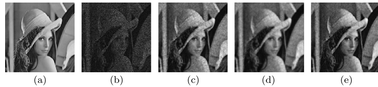
Fig. 15. Inpainting with the Lena image with Rayleigh noise: (a) original, (b) noisy image with 50% of the pixels missing; estimates using: (c) ATVF-1, (d) ATVFRW-1, (e) ADMM.
