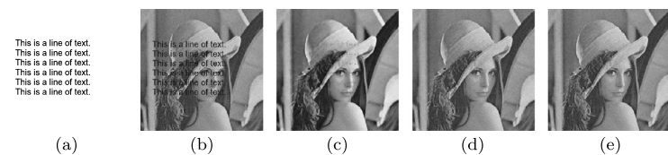
Fig. 8. Inpainting with the Lena image, Gaussian noise with superimposed text: (a) sampling mask, (b) observed image; estimates using: (c) ATVF-1, (d) SALSA, (e) FISTA.
