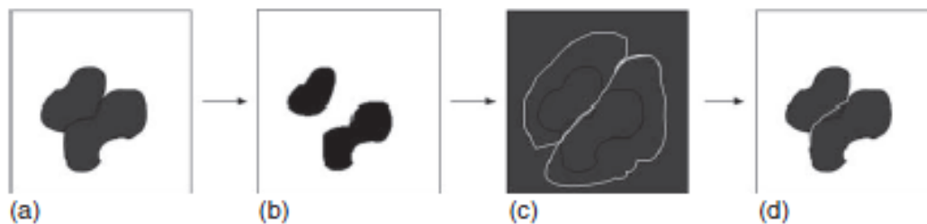
Figure 3.5: Illustration of separating touching objects. [3] (a) A binary segmented image. (b) After a few erosions and inversion. (c) The exoskeleton. (d) Separated objects
