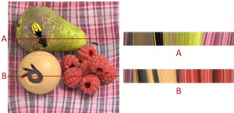
Fig. 1. Epipolar plane images obtained from slicing and stacking the sequence of viewpoint images at position A and B for the Still dataset [14].
