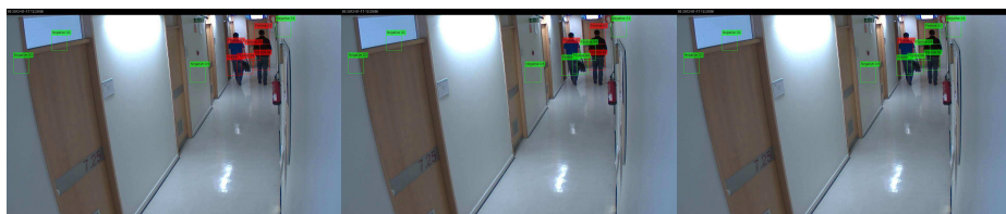
Fig. 3. Example of an instance classification using the MI-SVM classifier for increasing rate of positive instances on positive bags: 0.5, 0.7, and 0.9. The image regions in green correspond to instances correctly labeled while the image regions in red correspond to mislabeled instances.
