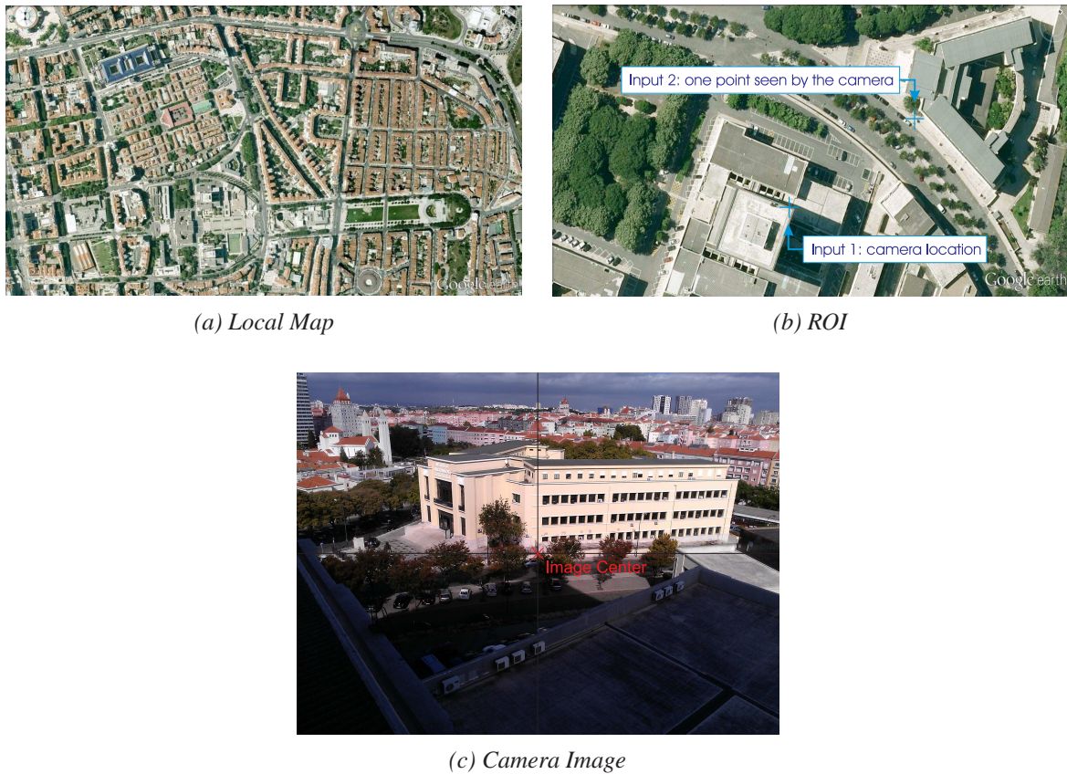
Fig. 1: Nominal calibration of a camera mounted in its operating place. The local map (a) is zoomed and cropped to a region of interest (ROI), for easier usage, where the camera location and a point seen by the camera (b) can be marked. This scene point is believed to be a point lying on the (camera optical axis), which projects (approximately) on the camera image center (c).
