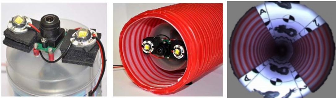
Fig.1: Tubular-Shape inspection setup. Camera equipped with wide angle lens (FOV > 180°) and illumination LEDs (left). Mockup tubular shape to inspect (middle). Captured image (right).
