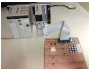
(b) Setup based on a single input and output module
