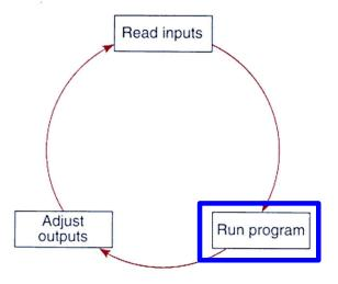
Adjusted outputs is what the hardware connected to the PLC see as IO and also what you see on screen.
