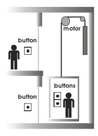
[Requests-buffer] The requests generated by the buttons are accumulated in a queue. Requests sorting is not considered in this problem. Just consider a simplified PN with incidence matrix  $D_1 = D_a$  where the place marking indicates the number of queued requests (pushed down buttons).
