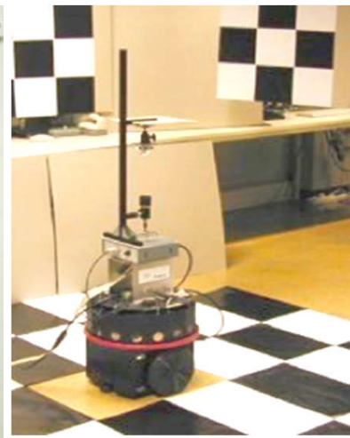
Micro-machined mirror, camera mounting, acquired images [IST/Portugal, USP/Brazil].
