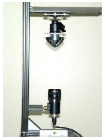
Micro-machined mirror, camera mounting, acquired images [IST/Portugal, USP/Brazil].
