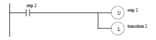
If step2 is active then it is going to be made inactive (unlatched). Note however that the code parts 1,2 and 3 run in a single scan cycle.
