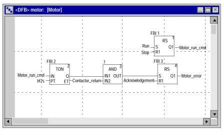
When Run = 1 and Stop = 0, the motor can be controlled (Motor\_run\_cmd = 1). The other part monitors the Contactor\_return variable. If Contactor\_return is not set to "1" after the Discrete counter counts two seconds, the Motor\_error output switches to "1".
