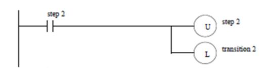
If step2 is active then it is going to be made inactive (unlatched). In Unity-Pro step2 gets inactive only after transposing transition2.
