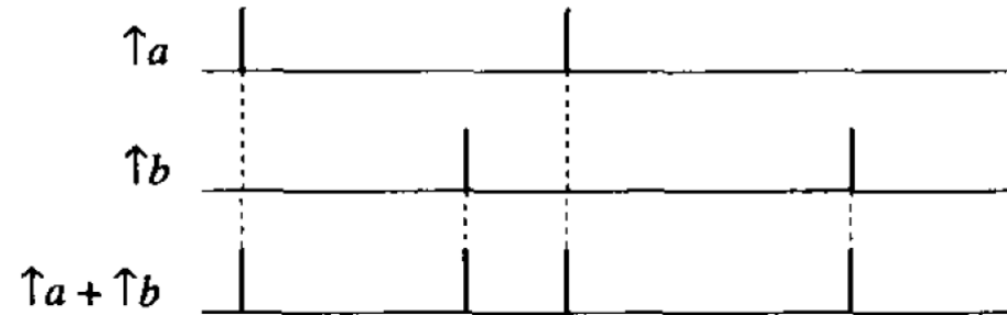
(d) Event \uparrow a + \uparrow b obtained from events \uparrow a and \uparrow b
