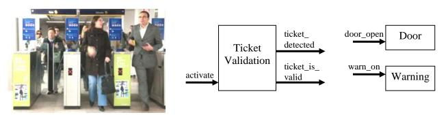
Figure 1: Main subsystems of an automated access system. List of inputs and outputs.
