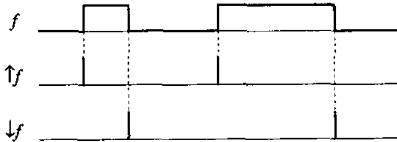
(a) Events \uparrow f and \downarrow f obtained from a condition f
