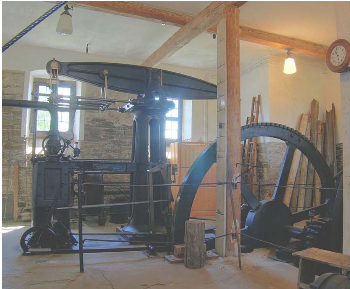
A steam engine built to James Watt's patent in 1848 at Freiberg in Germany [wikipedia]
