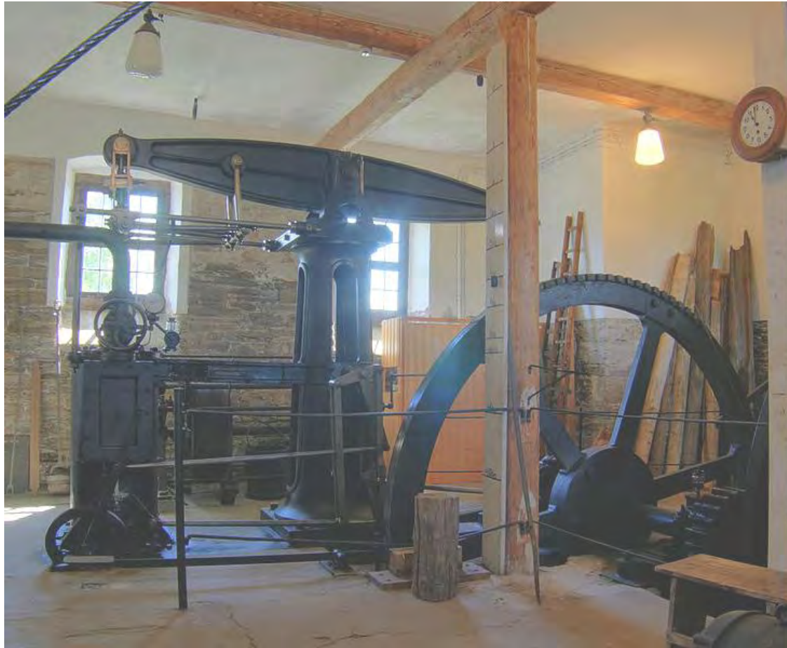
A steam engine built according to James Watt's patent in 1848 at Freiberg in Germany [wikipedia]
