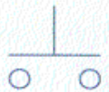
Normally open (NO) pushbutton
