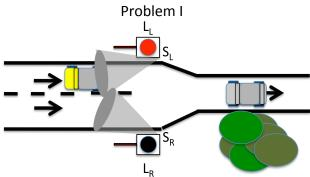
This problem will focus on the modeling and synthesis of a discrete event system: an automatic traffic light system must be installed on the confluence of two roads that give access to a narrow way, as depicted in the above figure. There are two sensors  $S=\{S_L, S_R\}$ , with binary outputs to detect the presence/absence of vehicles in the left and right way, respectively. There exists also installed two red lights  $A=\{L_L, L_R\}$ , one at each side, both with a digital ON/OFF command.
