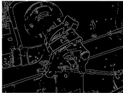
(c) Result of Canny edge detector.
