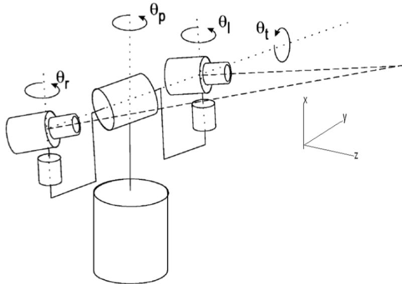
Figure 3.3: Scheme of Baltazar robotic head, code-named “Medusa” [BSV99]. The meaning of the four joint angles  $\theta_l$ ,  $\theta_r$ ,  $\theta_p$  and  $\theta_t$  is explained in Table 3.1.
