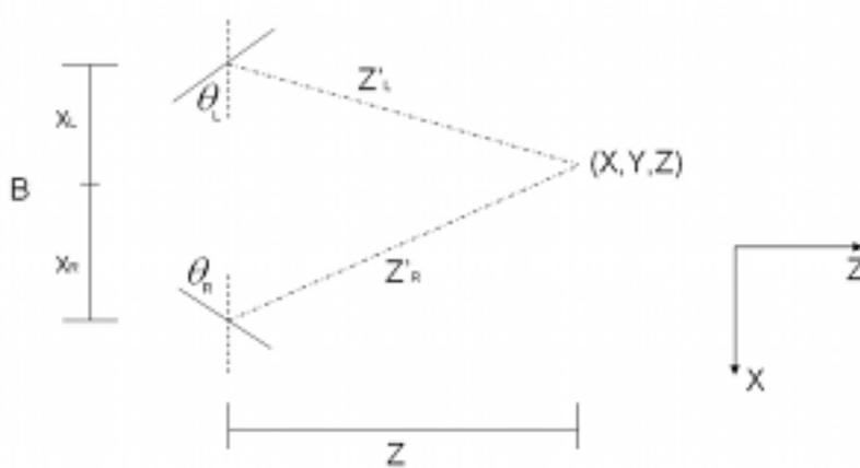
Figure 4.5: 3D reconstruction scheme for a stereo pair of cameras with arbitrary vergence.
