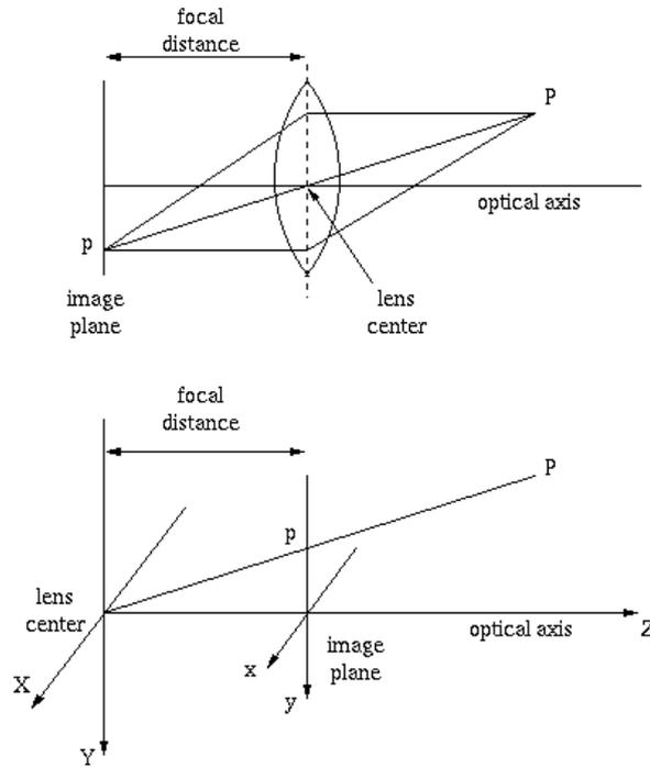
Figure 4.4: Pinhole camera model.
