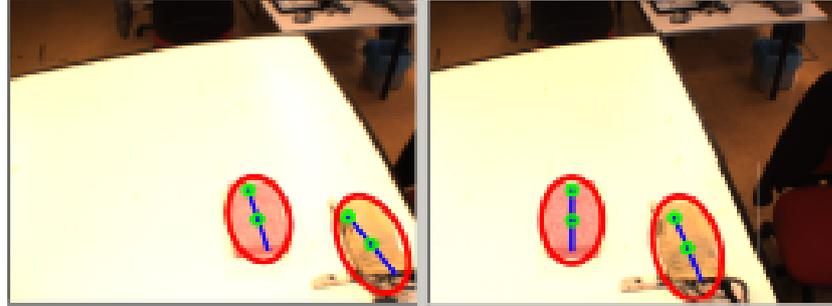
(a) Object and hand are parallel;  $\mathbf{u} = (X = -0.006, Y = -0.062, Z = -0.041), \theta = 4.285^\circ$ .
