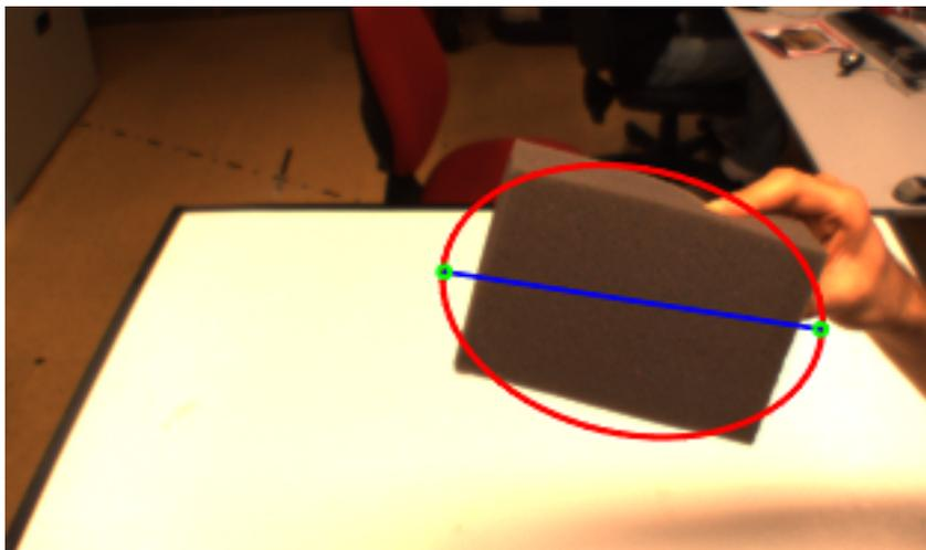
Figure 5.1: CAMSHIFT tracking experiment, with a grey sponge.
