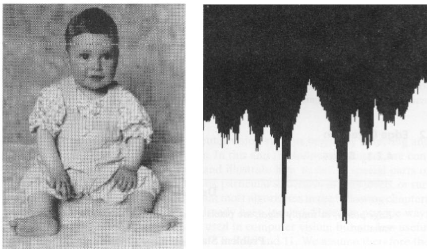
(a) A  $325 \times 237$ -pixel image, with scanline  $i = 56$  (over the baby's forehead) highlighted. (b) Intensity profile along the highlighted scanline.
