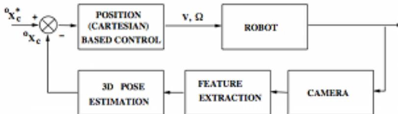
Figure 2.18: Block diagram of PBVS [HHC96]. The estimated pose of the target,  ${}^c\mathbf{x}_0$ , is compared to the desired reference pose,  ${}^c\mathbf{x}_0^*$ . This is then used to estimate the velocity screw,  $\dot{\mathbf{q}} = [\mathbf{V}; \mathbf{\Omega}]^T$ , for the robot so to minimize the error.
