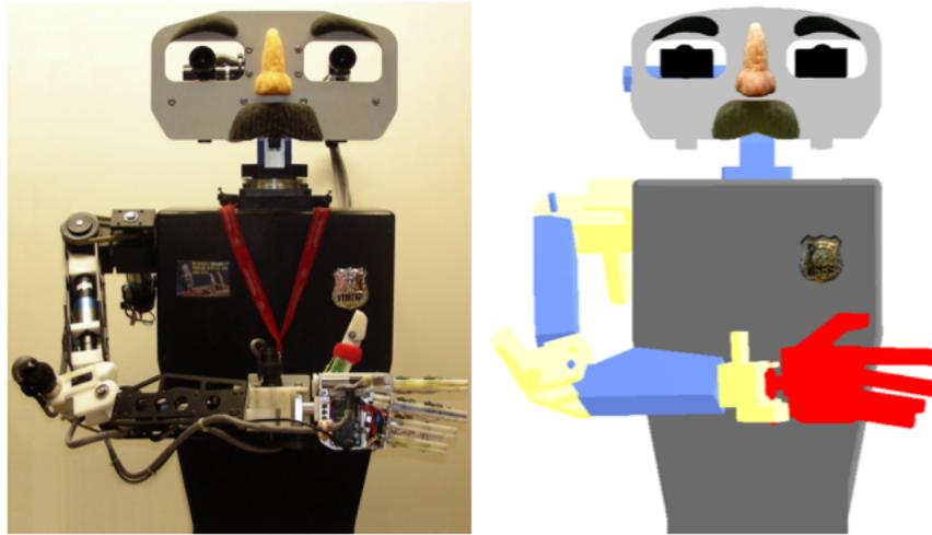
Figure 3.5: Real Baltazar and its CAD model (obtained with the Webots robot simulator [Web]).
