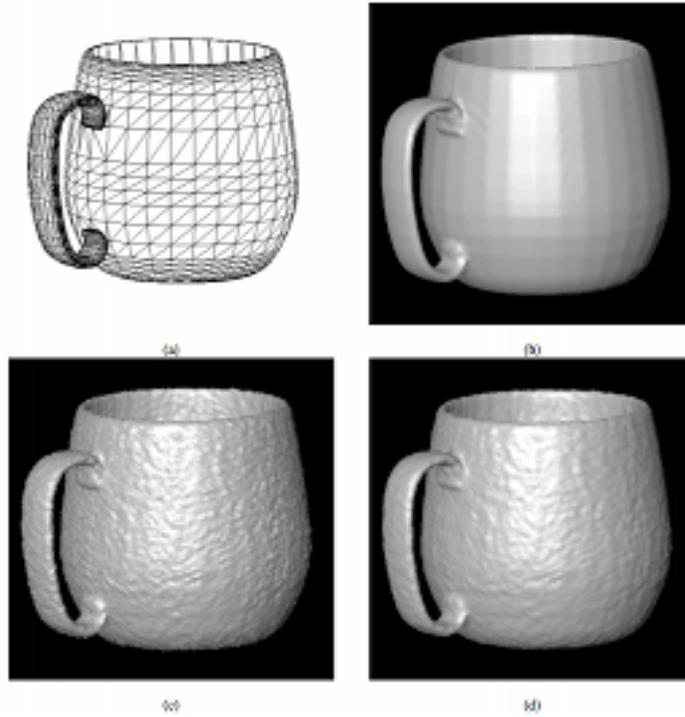
Figure 2.9: Level set based 3D reconstruction of a mug, using synthetic data generated from a 3D model (a). Without noise, the reconstruction (b) is limited only by the resolution of the model,  $140 \times 140 \times 140$ . With noise, the surface appears rough (c). Including a prior improves the appearance of the reconstruction (d).
