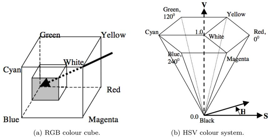
Figure 4.2: RGB and HSV colour spaces. In the single-hexcone HSV model, the  $V = 1$  plane contains the RGB model's  $R = 1$ ,  $G = 1$ , and  $B = 1$  planes in the regions shown.
