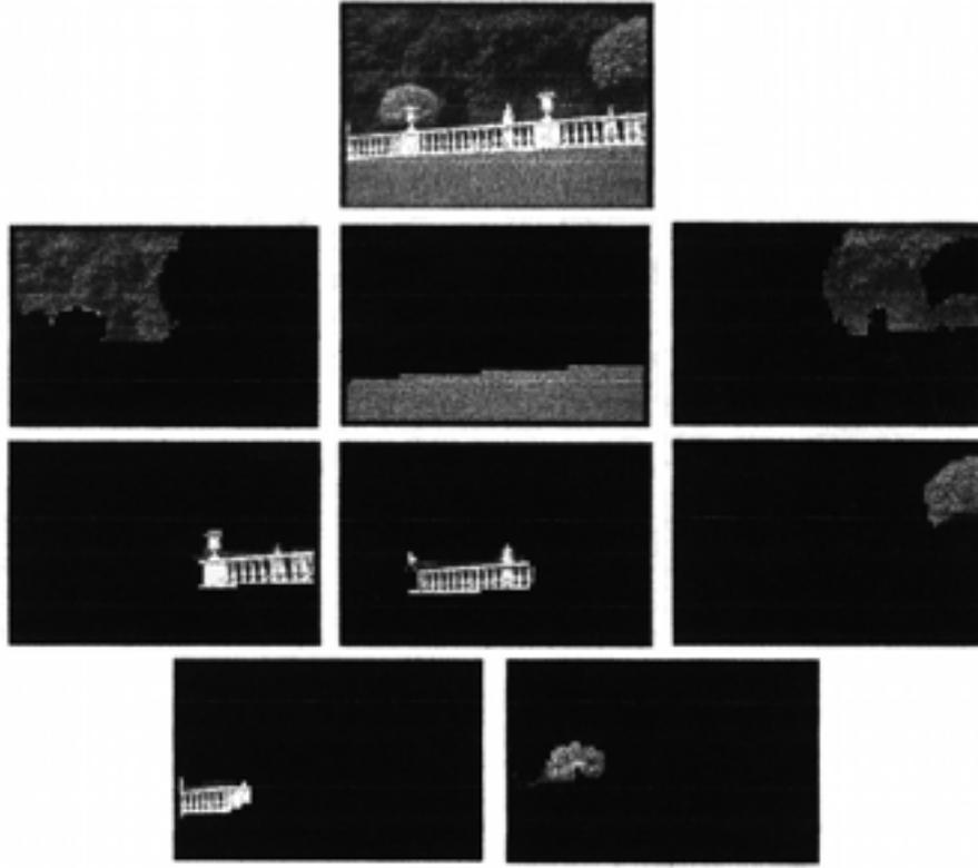
Figure 2.6: The image on top being segmented using the normalized cuts framework into the components shown below. The affinity measure used involved both intensity and texture. Thanks to having a texture measure, the railing shows as three reasonable coherent segments, which would not have happened with other approaches such as  $k$ -Means.
