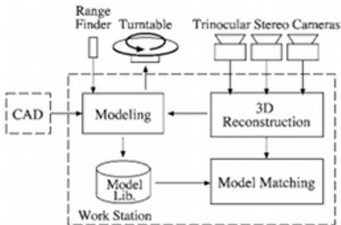
Figure 2.1: Block diagram of the “VVV” 3D vision robot system [SKYT02].
