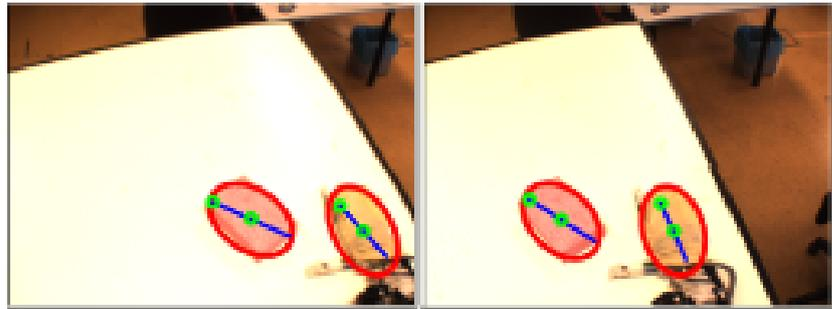
(b) Object and hand have a relative slope of roughly  $45^\circ$ ;  $\mathbf{u} = (X = -0.129, Y = 0.737, Z = -0.129), \theta = 49.413^\circ$ .
