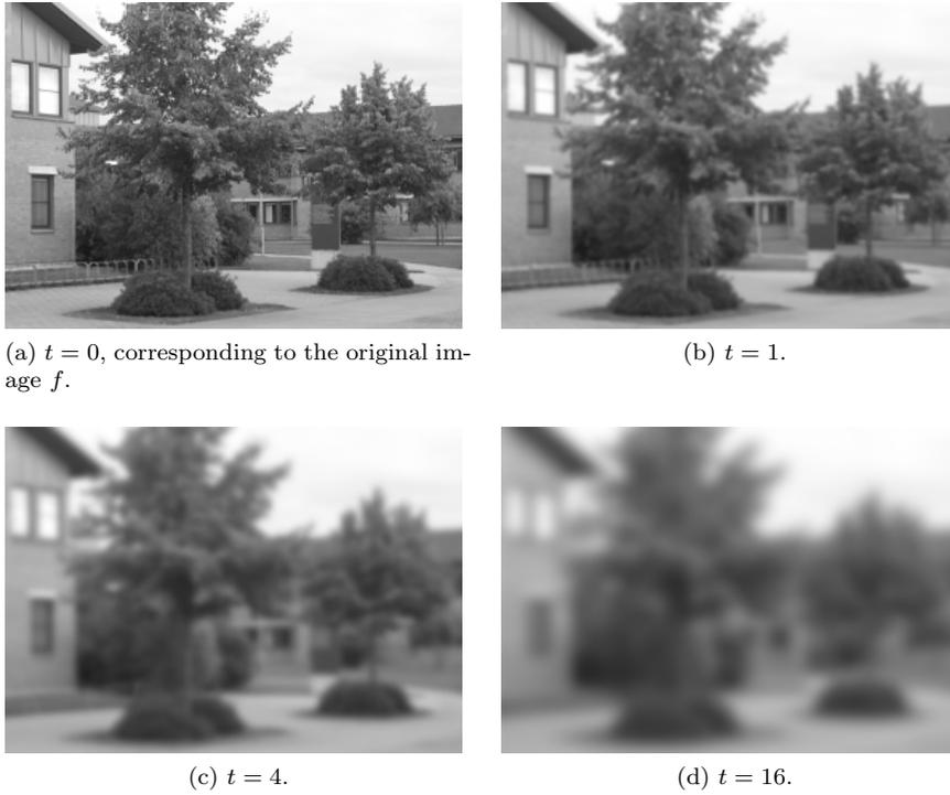
Figure 2.13: Space-scale representation  $L(x, y; t)$  for various  $t$  scales. As the parameter  $t$  increases above 0,  $L$  is the result of smoothing  $f$  with a larger and larger filter.
