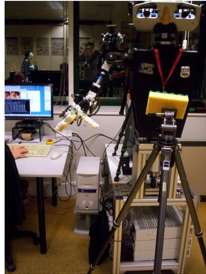
(b) Robot arm is now within the field of view of cameras.
