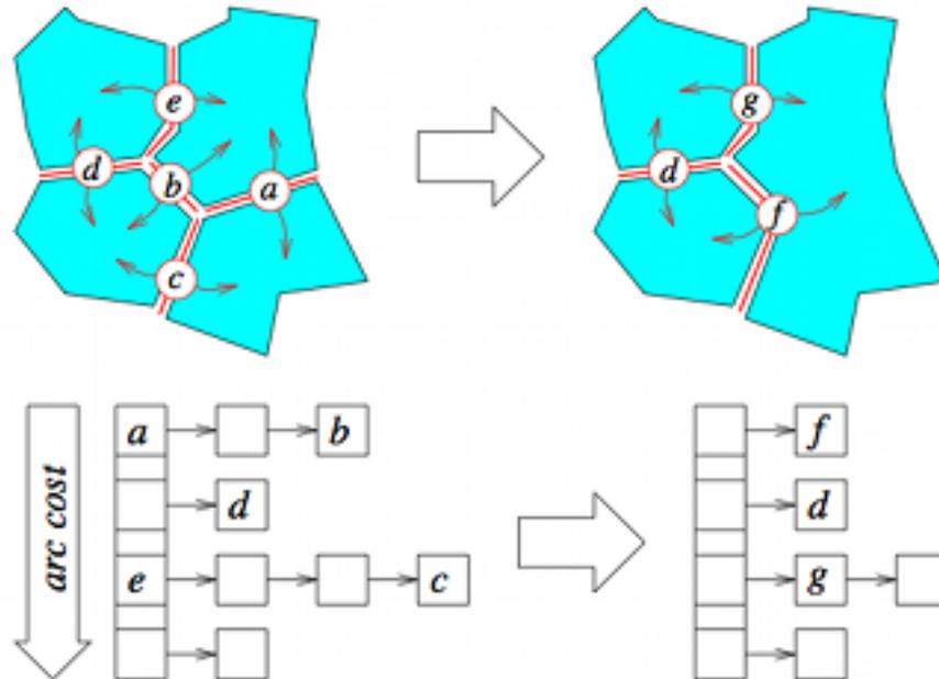
Figure 2.12: One iteration of the region growing process during which the two patches incident on the minimum-cost arc labelled *a* are merged. The heap shown in the bottom part of the figure is updated as well (which bears a considerable computational cost): the arcs *a*, *b*, *c* and *e* are deleted, while two new arcs *f* and *g* are created and inserted in the heap.
