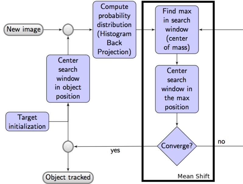
Figure 4.1: Block diagram of CAMSHIFT.
