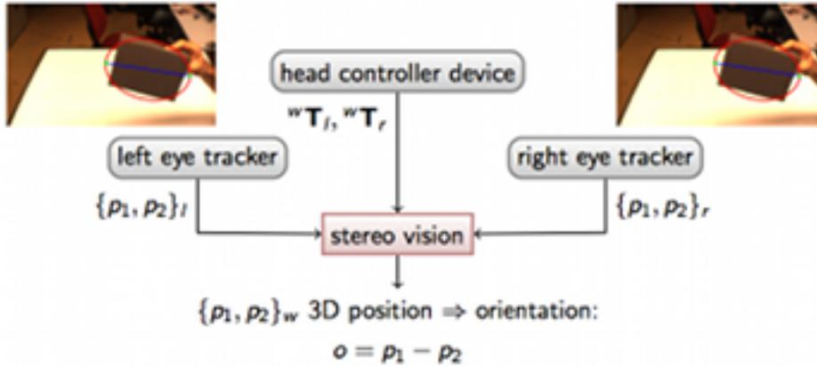
Figure 4.6: 3D reconstruction software module scheme, outlining the data that are passed as inputs/outputs among YARP modules.
