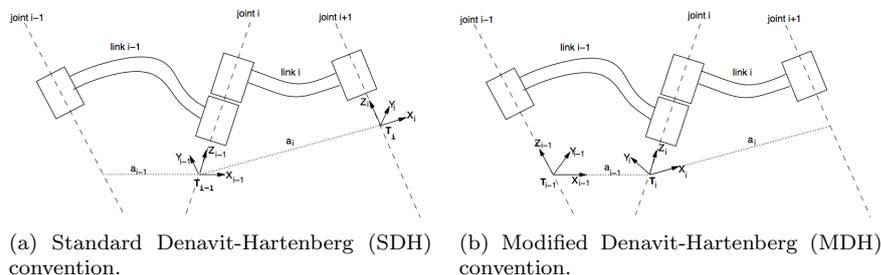
Figure 3.2: Different forms of DH notation. Note:  $a_i$  always indicates the length of link  $i$ , but the displacement it represents is between the origins of frame  $i$  and frame  $i+1$  in the standard form, between frames  $i-1$  and  $i$  in the modified form.
