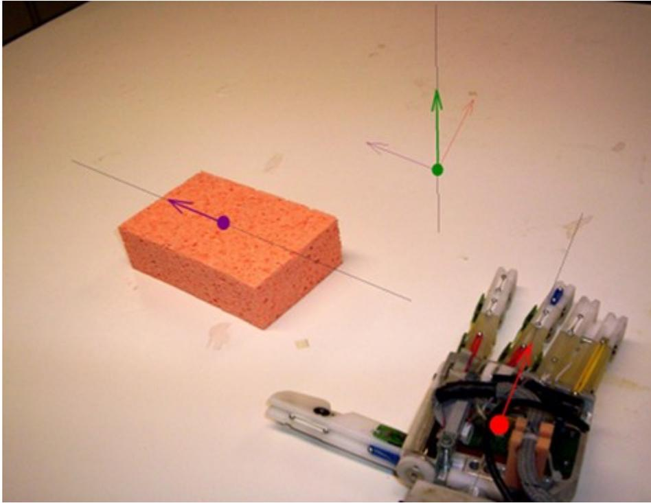
Figure 4.8: Unit vector of the target object along its orientation axis (purple); unit vector and orientation of robot hand (red); third axis resulting from their cross product, and corresponding unit vector (green).
