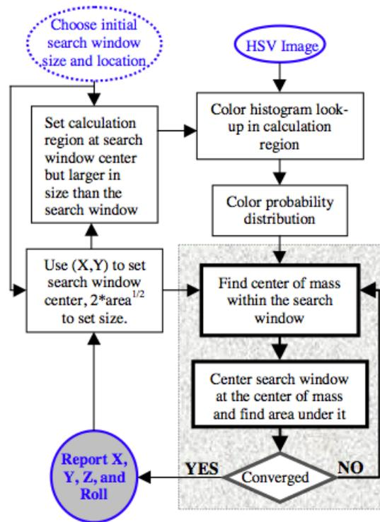
Figure 2.7: Block diagram of histogram-based object tracking. The grey box is the Mean Shift algorithm.
