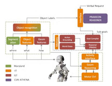
Figure 62: POETICON++ project software architecture. The contributions by IST are marked in red.
