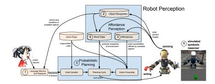
Figure 52: POETICON++ architecture exposing the main components of our system. In the bottom left, a human user expresses an instruction in natural language. In the bottom right, a robot reasons about the environment and executes the instruction. The robot can be real or simulated. The components (software modules) of the system are represented as gray rectangles, or gray cylinders in case they incorporate a knowledge base. Arrows indicate data flow.
