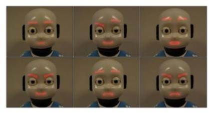
Figure 75: A set of iCub facial expressions using eye LEDs, mouth LEDs and eyelid motors.
