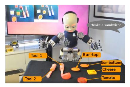
Figure 55: Example of the initial state of the sandwich making problem. The instruction provided by the human is reported in the gray balloon, the objects are annotated with orange boxes, and the output of the visual perception routines is shown in the back screen. Note that perceiving the affordances of tools does not require their names.
