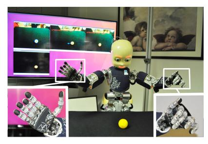
Figure 41: The iCub humanoid robot performing motor actions with different hand postures onto a physical object. In the background screen, we show the visual routines that monitor the evolution of the environment.
