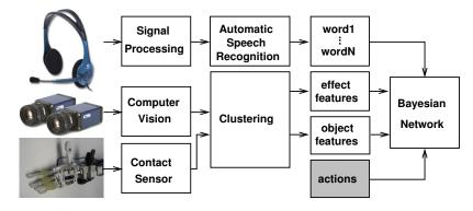
Figure 12: Experimental setup of [Sal+12]. In this work, which extends [Mon+08], a robot learns associations between *spoken* words and object affordances (where affordances are modeled as the relationships between actions, object features, effect features).
