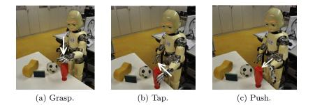
Figure 19: Examples of manipulative motor actions performed by the iCub robot onto environment objects.
