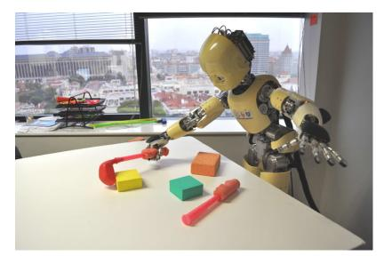
Figure 18: The iCub robot in a playground table scenario. Objects and tools are present in the scenario, so that the robot can interact with them, it can acquire a model of the environment derived from sensorimotor data, and it can use such a model for reasoning about the environment.
