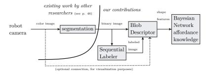
Figure 20: Our pipeline for computing visual affordance features. Boxes indicate software modules, arrows indicate data flow connections, dotted arrows indicate optional data flow connections. See text for details, and Fig. 21 for an example computation.
