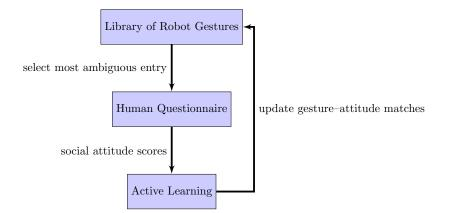
Figure 77: Block diagram of the proposed approach to study the matches between robot gestures and perceived social attitude in humans. The library of gestures is pre-programmed (see Table 18); the questionnaire is a multiple-scale Likert one; the scores are numbers corresponding to the Likert answers, and they are used by the Active Learning block to update an internal matrix of matches and select which robot gestures should be shown next.
