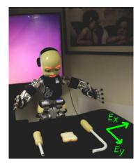
Figure 37: The iCub robot in a tool use scenario, with green overlay arrows showing the effects (i.e., displacements of objects).
