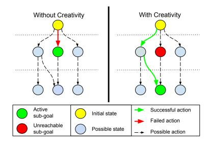
Figure 53: Creativity heuristic. Each row represents a temporal step. When no action is found for a certain sub-goal, and the planning horizon is already too large, this heuristic allows the planner to jump to the next sub-goal and attempt that one instead, bypassing deadlocks.
