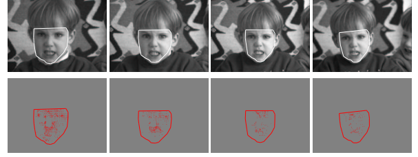
Figure 6. Real image deformations approximated by an affine deformation. The first column shows the model, and the remaining images present the deformed model contour using the affine transform computed using the matches depicted on the second rows as the red dots. The whole sequence contains 30 images.
