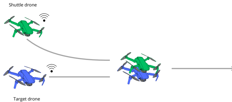
Figure 1.1: Cooperative capture manoeuvre between two quadrotors
