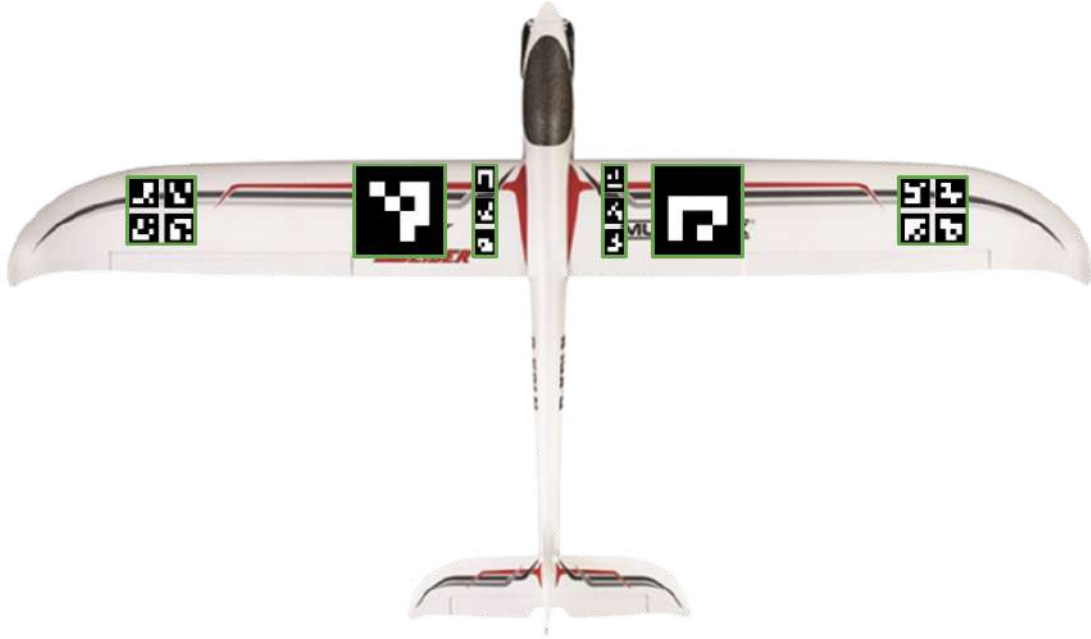
Figure 36: Example of ArUco boards disposal on the target drone.
