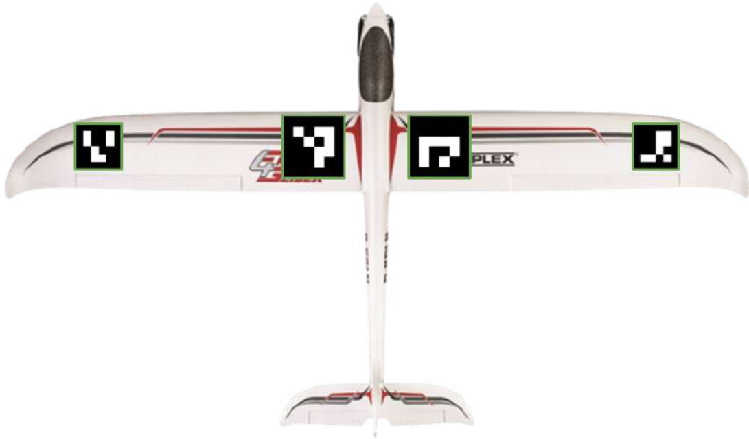
Figure 40: New configuration of ArUco boards on the target drone.
