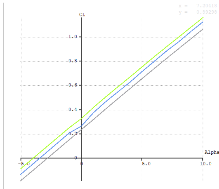
Figure 4.4: Coefficient of lift in function of alpha. Grey line- negative elevator deflection, Blue line- neutral configuration , Green line - positive elevator deflection.
