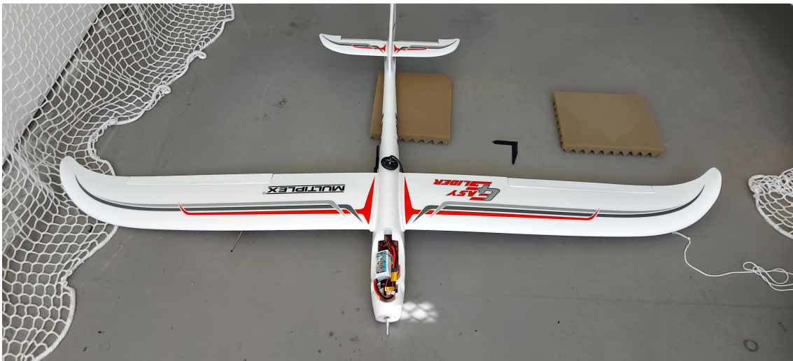
Figure 3.6: Up view of the easy glider with all the hardware assembled.
