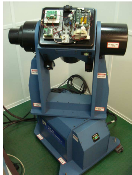
Fig. 9. Experimental setup mounted on the Ideal Aerosmith motion rate table.
