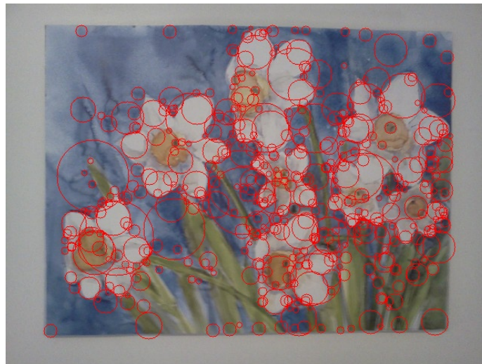
Figure 3.2: An example of the type of features that the Fast Hessian Detector detects
