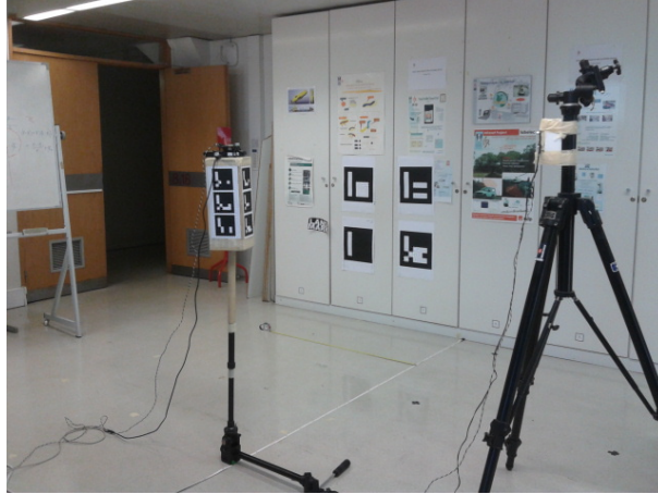
Figure 4.20: Final experimental set-up, with Cricket beacon nodes, visual tags and the target comprising a Cricket listener and a camera
