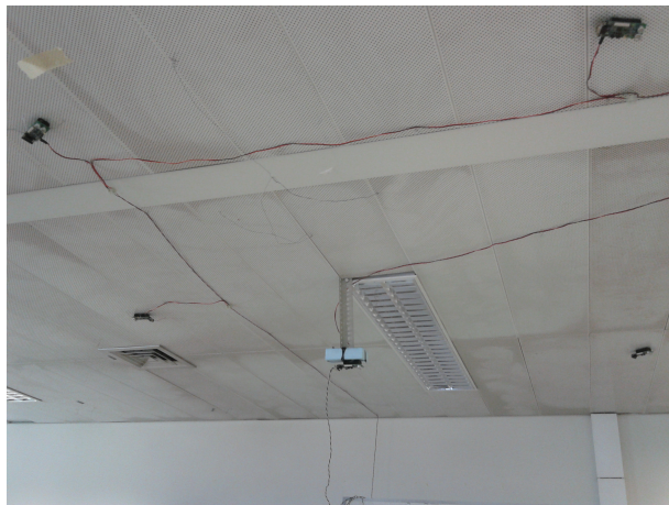
Figure 4.14: Cricket beacons attached to the ceiling in the first experimental set-up
