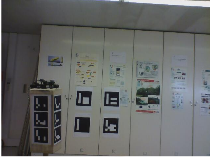
Figure 4.33: View from sensor 2 camera, showing sensor 1 and the visual tag
