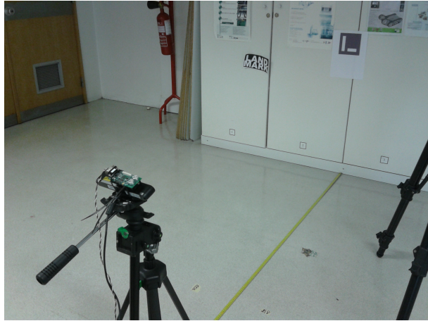
Figure 4.13: Testing the first prototype, consisting of a Cricket listener mounted on a camera
